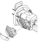
These reduce the flow of cooling air and prevent large amounts of snow from being sucked into the carburetor space.
